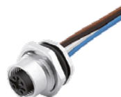
Female panel mount connector, rectangular flange, with single wires, metal housing, IP40 without sealing, IP67 with sealing (16 0959 000)
