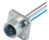
Female panel mount connector, rectangular flange, with single wires, metal housing, IP40 without sealing, IP67 with sealing (16 0959 000)
